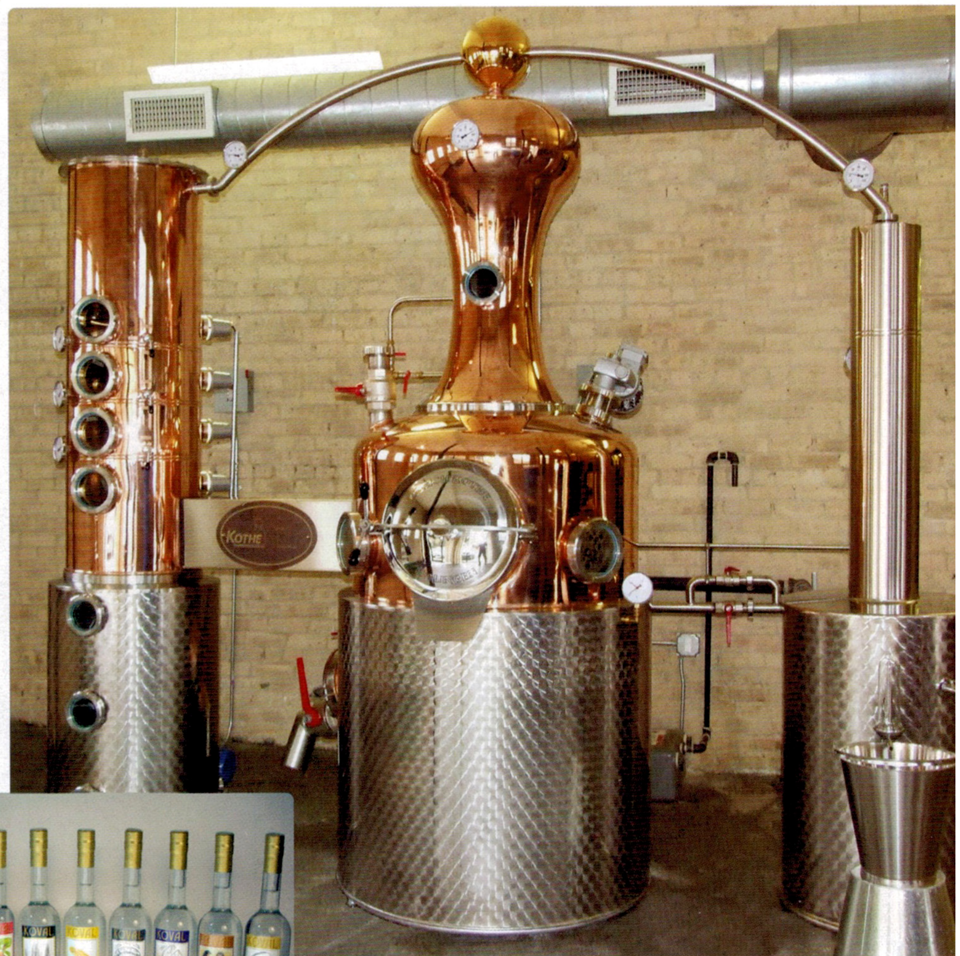
Above: The Koval Kothe still arrangement complete with super aromator and super dephlegmator.
